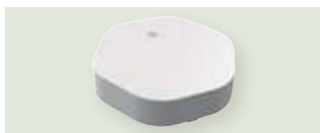
Water leakage sensor. Two sensing pads under the body activate when water is present between the two pads. Detecting the water, the sensor reports the event to the controller (and BEMS).
