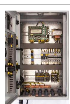
**Q4E – ELECTRICAL PANEL FOR EC FANS WITH PAINT COATED** METAL CASING, INTERNALLY MOUNTED CONTROLLER, PROTECTED BY AUTOMATIC SWITCHES (CIRCUIT BREAKERS) CONNECTED TO GROUPS OF FANS, FAN REGULATION CONTROL MODBUS RS485. PANEL-MOUNTED SWITCHES (1 SWITCH EVERY 2 FANS) (1X2).
