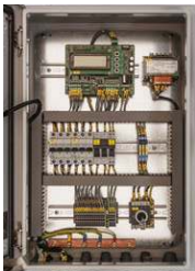
Q2E - THREE-PHASE ELECTRICAL PANEL FOR 400V-3-50HZ EC FANS Electrical panel for EC fans with paint coated metal casing, controller mounted inside the box, protected by automatic switches (circuit breakers) connected to groups of fans, fan regulation control MODBUS RS485.
