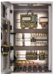
Q4E - THREE-PHASE ELECTRICAL PANEL FOR 400V-3-50HZ EC FANS Electrical panel for EC fans with paint coated metal casing, controller mounted inside the box, protected by automatic switches (circuit breakers) connected to groups of fans, fan regulation control MODBUS RS485. Panel-mounted switches (1 switch every 2 fans) (1x2).
