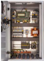
Q3E - THREE-PHASE ELECTRICAL PANEL FOR 400V-3-50HZ EC FANS Electrical panel for EC fans with paint coated metal frame, controller mounted inside the box, protected by automatic switches (circuit breakers) connected to groups of fans, fan regulation control MODBUS RS485, internal anti condensate heating element.
