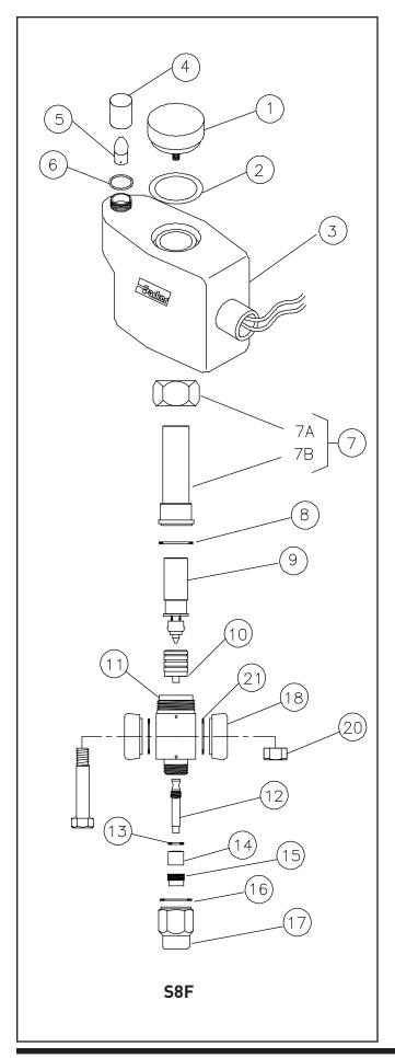
Solenoid Coil is de-energized, allowing #9 Solenoid Plunger to drop and Valve Needle to close the Pilot Port in #10 Piston Plug. Liquid and/or gas leakage through the clearance area around #10 Piston Plug causes a rapid pressure build up in Chamber A which combines with the downward force of the Spring which is part of #9 Solenoid Plunger and the weight of #10 Piston Plug Assembly to force the Main Valve Disc tight against the Seat Bead to stop all flow.
