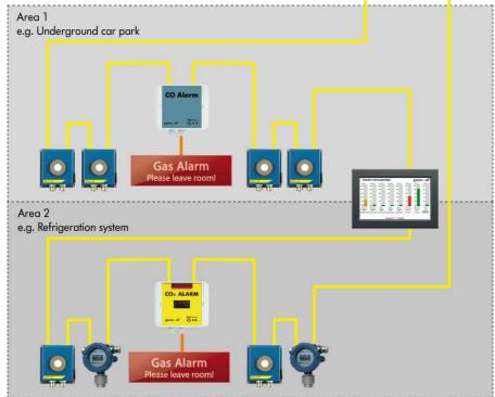
Alarm component-Wiring: 24 VDC or 230 VAC
