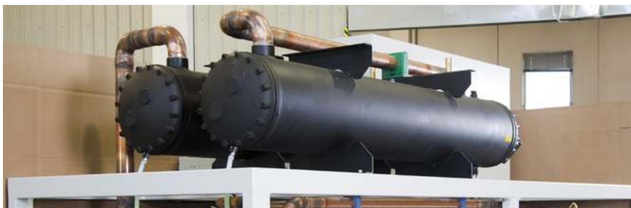
Condensatore fascio tubiero - Shell and tube condenser
