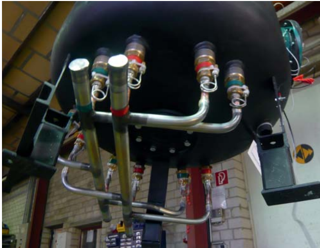
DK-HEAT RECOVERY with internal safety heat exchangers
