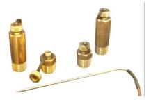
The "Test Plugs" probe, also called "binder probes", offers an excellent solution to get high accuracy and quick response as the sensor is inserted in the flow. They eliminate the temperature pockets that delay response and create a risk for freezing at low temperature and the sensors can easily be removed for calibration. Type C - Probe is 150 mm long with 3 mm diameter with an angle to give a good hold when it is inserted or removed.
